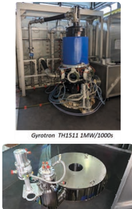
Figure 1: ECRH components being tested at KIT
