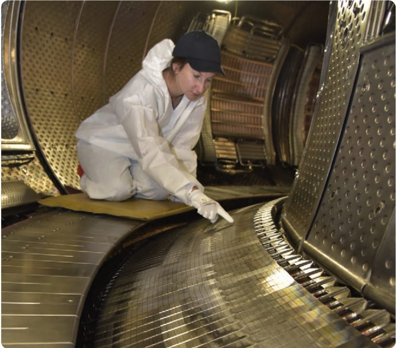
Figure 3: New ITER-technology solid tungsten components from the WEST divertor
