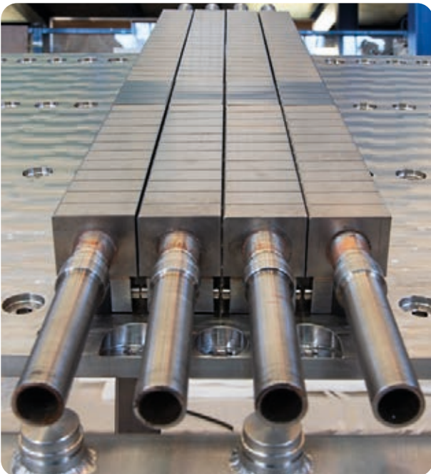
Figure 3. Elements of the actively cooled divertor in WEST. Each Plasma-Facing Unit (PFU) is equipped with 35 tungsten monoblocks. The WEST divertor has 456 PFUs. The luminosity differences reproduce the variable shapes, bevels and angles of the monoblocks.
