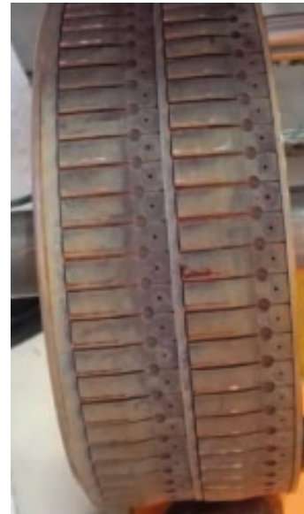
Figure 3: RF contacts after testing at 1.5 kA for 3,600 s.
