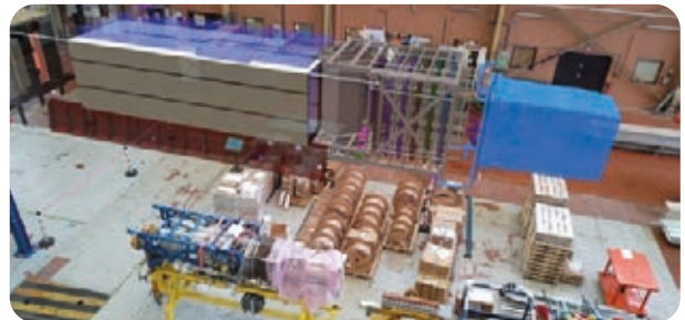
Figure 3: Simulation of the installation of a scale 1 TBS mockup in a hall at DRF/IRFM. In the foreground, a heating antenna of the WEST tokamak and its auxiliaries illustrate the scale factor between a WEST component and an ITER component.
