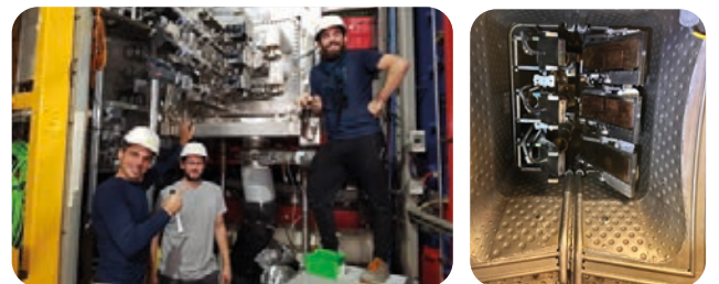
Figure 3: ECRH antenna assembled in the tokamak with its three channels
