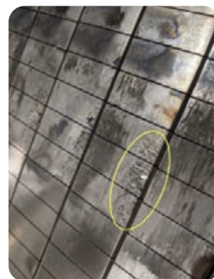
Figure 5: visual inspection of the WEST ITER grade divertor after the High Fluence campaign. Left: picture of divertor sector Q4A (PFU 1 to 19), showing the main features observed after the High Fluence Campaign. The position of the outer/inner strike point during the High Fluence campaign is indicated (OSP/ISP respectively), as well as the position of shadowed areas by bevels. Thick deposits on the High Field Side (HFS) are also indicated. Right: zoom on thin foil like deposits found in the areas shadowed by the toroidal bevel of the ITER grade PFU.
