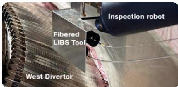
Figure 1: LIBS installed on the Articulated Inspection Arm
