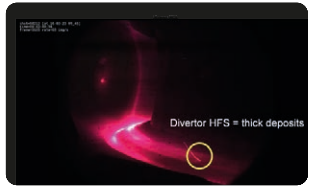
Figure 4: illustration of UFO detected during the High Fluence campaign, evidenced as peaks on the radiated power (left) or observed in the visible camera field of view, starting from the divertor High Field Side (HFS), which is an area with thick-deposited layers (right).
