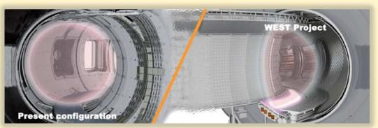
operation of the ITER tungsten components emerge truly as a "first" in the world. They create new challenges that the WEST (acronym derived from W Environment in Steady-state Tokamak, where W is the chemical symbol for tungsten) Project will be able to meet.
