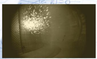
Impact of a runaway beam on the WEST inner wall limiters. Tungsten dust heated and ablated by the beam is seen flying off the tiles.
