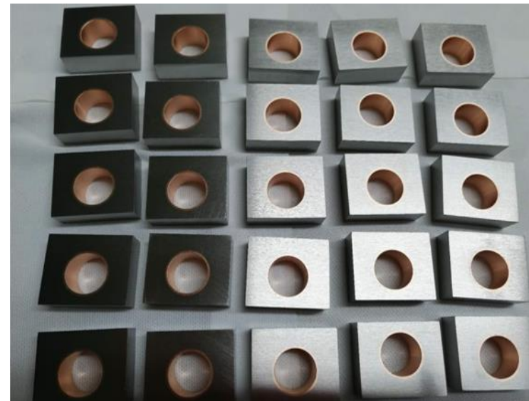
Blocks W/Cu after machining and UT
