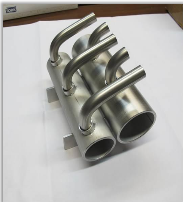
Prototype for welding validation
