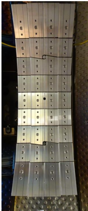
Outer limiter with massive W tiles
