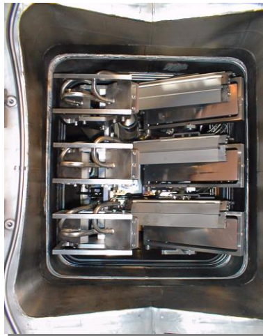
ECRH antenna with actively cooled mirrors
