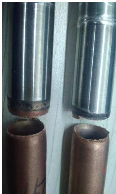
Tube-to-tube transition tensile test
