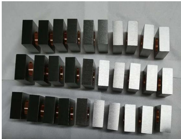
Blocks W/Cu after machining and UT
