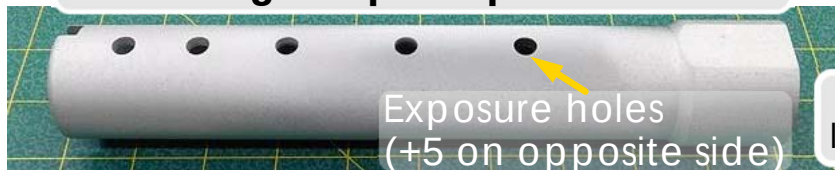
Samples show surface deposition due to exposure; Analysis on-going to determine deposit composition
