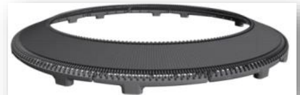
Phase 2: high heat flux & fluences on 360° actively cooled ITER like divertor
