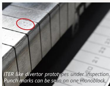
ITER like divertor prototypes under inspection. Punch marks can be seen on one monoblock.
