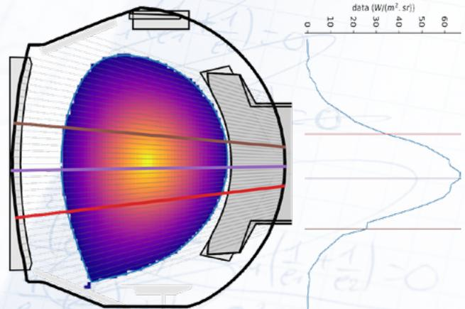
Tomographic reconstruction of SXR intensity in a WEST poloidal cross section (left) with a synthetic field peaked on the magnetic axis and all three highlighted LOS of the SXR diagnostics (right) corresponding to LOS-integrated signal.
