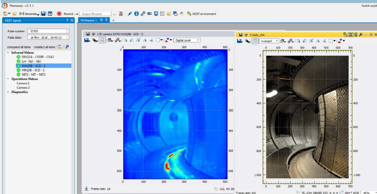
Thermal scene from C3 experimental campaign in July 2018 showing the heat load on the lower divertor target and spurious hot spots (reflections) during the plasma.
