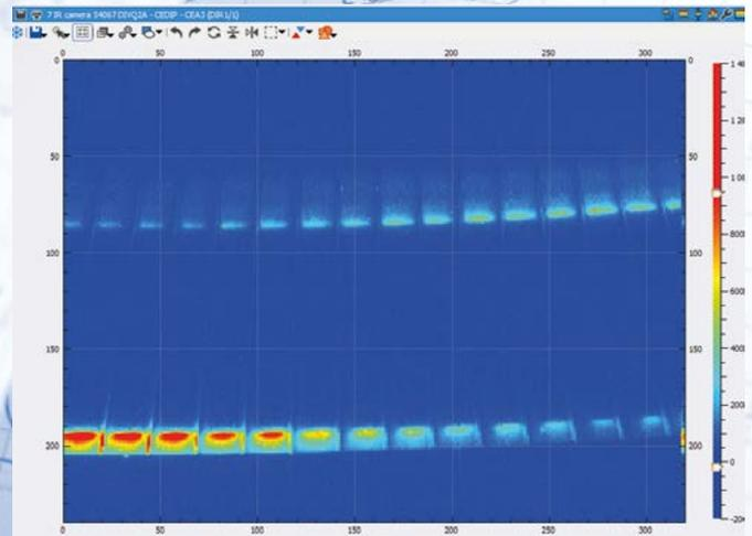
IR emission from the WEST divertor during plasma experiment showing the heat fluxes on the tungsten coated plasma facing units.
