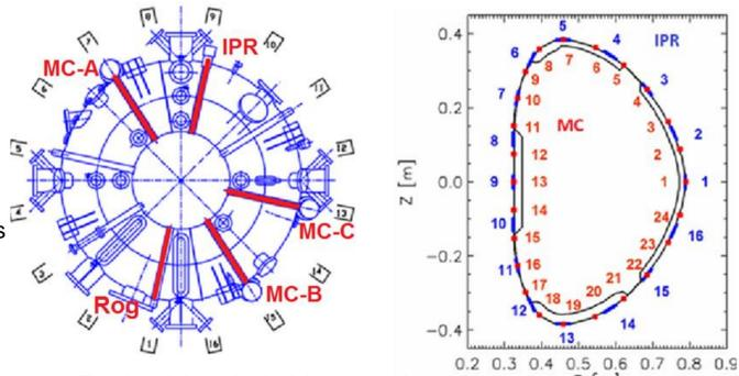
Top view (left) and poloidal cross-section (right) of the COMPASS tokamak showing location of magnetic diagnostics
