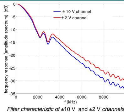
Filter characteristic of ±10 V and ±2 V channels
