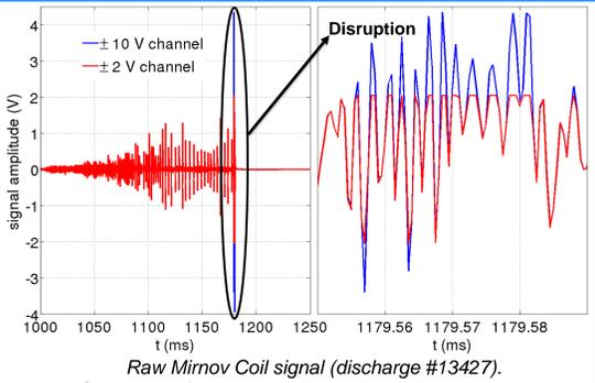
Raw Mirnov Coil signal (discharge #13427). Saturation of ±2 V channel raw signal during disruption
