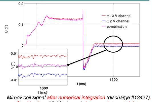
Mirnov coil signal after numerical integration (discharge #13427). Combination of DAQ channels improves integrated data.
