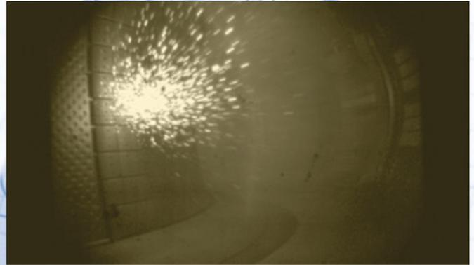
Impact of a runaway beam on the WEST inner wall limiters. Tungsten dust heated and ablated by the beam is seen flying off the tiles.
