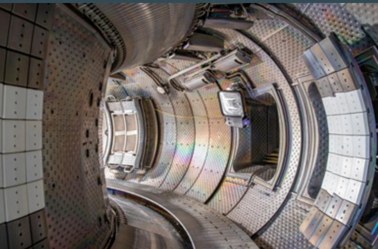
White components are the boron nitride tiles that replace the tungsten tiles on WEST inner and outer limiters for the next experimental campaign.
