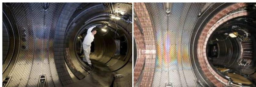
components like the Toroidal Pumped Limiter and the CFC carbon tiles of the inner bumpers were disassembled.
